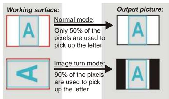
Picking up a complete vertical (portrait) letter or A4 page has always been a critical issue for a video camera based system, because the image is always picked up in a horizontal (landscape) format. **Progressive Scan** cameras handle this task much better, because of the improved resolution.
